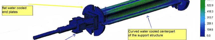
Position of engine for motor drive not drawn support roll. Here four engines are attached to the support structure
