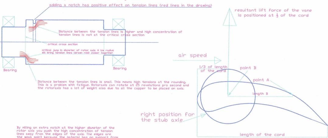
By milling an extra notch at the higher diameter of the rotor axis you push the high concentration of tension lines away from the edges of the axis. The edges are the weak point because the material has no support from surrounding material. Air will not help supporting the axis. The notch will lower the high tensions in the critical diameter. As a consequenz the tensions will rise a little in the not critical part of the axis. The total product is now made much stronger.
