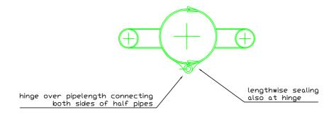
CONCEPT CONSISTS OF TWO HALF PIPES TO BE PLACED ON TOP OF LEAKING BOP. TUBES CAN HINGE.
